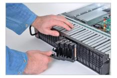
**Tool-less Easy Swap** Replace & secure your drives lightning fast with the flip of a button.
